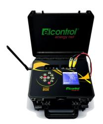
NanoVIP® BOX<sup>™</sup> does not require an external power source as it is self-powered by the same measurement line and equipped with a battery that allows it to remain active even in the absence of line for over 24h. 4G communication allows it to be fully controlled through direct SMS commands, send data to the Elcontrol Cloud or be fully remotely driven.
