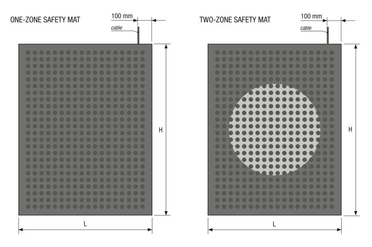
The safety mat is equipped with a 4-pole, FROR 300/500, outlet cable (4x0.35mm2) – standard length 3 m - placed at a distance of 100 mm from the right edge.
